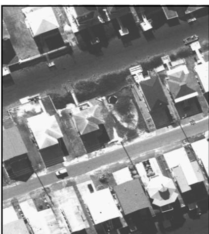
One of McQueen's vacant lots (note oval-shaped scarp line) in the center of this photo showing the effects of erosion. Also, see fully-bulkheaded lot at left center of photo.
